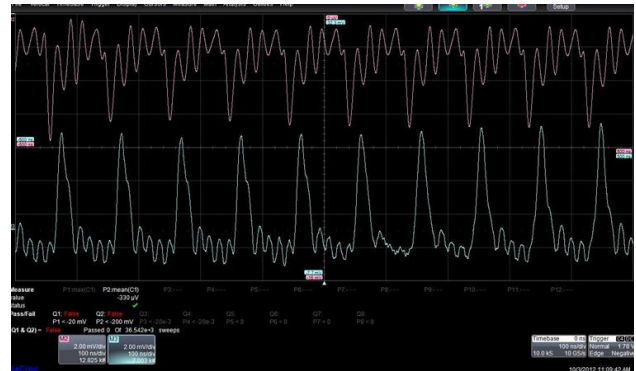
Figure 7: The time structure of MCP1 (upper signal) and photodiode (lower signal).
