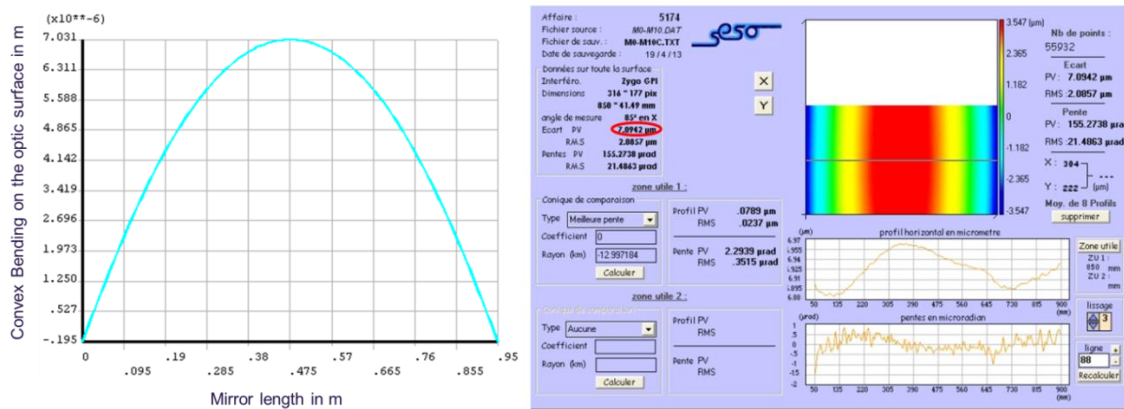
Figure 3. Bending profile of the optic surface: ANSYS result (left) and interferometer measurement performed by SESO (right)
